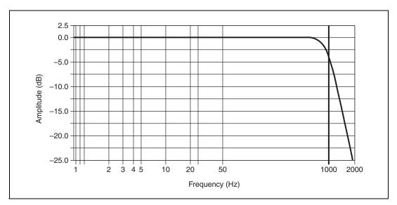
Figure 5. Typical SCC-LP04 Response Curve
